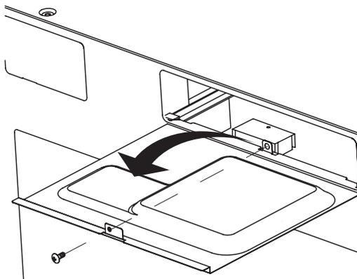
5. Remove burnt out LED light and replace only with an equivalent 1.5 watt LED light available from parts distributor, the part number is 5304499540.
