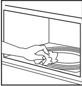
Use only mild, nonabrasive soaps or a mild detergent. Be sure to keep the areas clean where the door and oven frame touch when closed. Wipe well with clean cloth.
