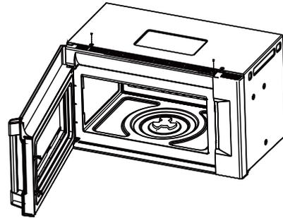
3. Slide the vent left and tip forward. Lift out to remove.
