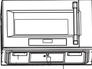
3. Soak grease filter in hot water and a mild detergent. Scrub and swish to remove embedded dirt and grease. Rinse well and shake to dry. Do not clean filter with ammonia, corrosive cleaning agents, such as lye-based oven cleaners, or place them in a dishwasher. The filters will turn black or become damaged.
