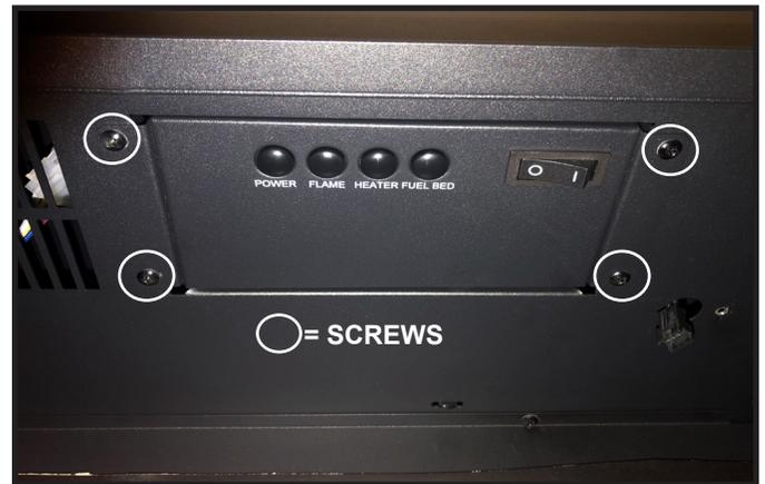
Figure 4 Control Board Location
