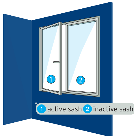
In case of double-leaf elements, the active sash must always be opened first (except escape doors) to avoid damage to the lock or frame.
